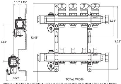
\*When extending the manifold, Viega requires using thread sealant paste on the 1"NPT manifold end connection.
